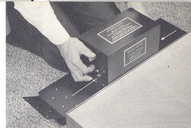
Figure 1: Installing the power supply on the terminal board at the base of the panel. Both locating pins (indicated by arrows) should be engaged at the same time.
