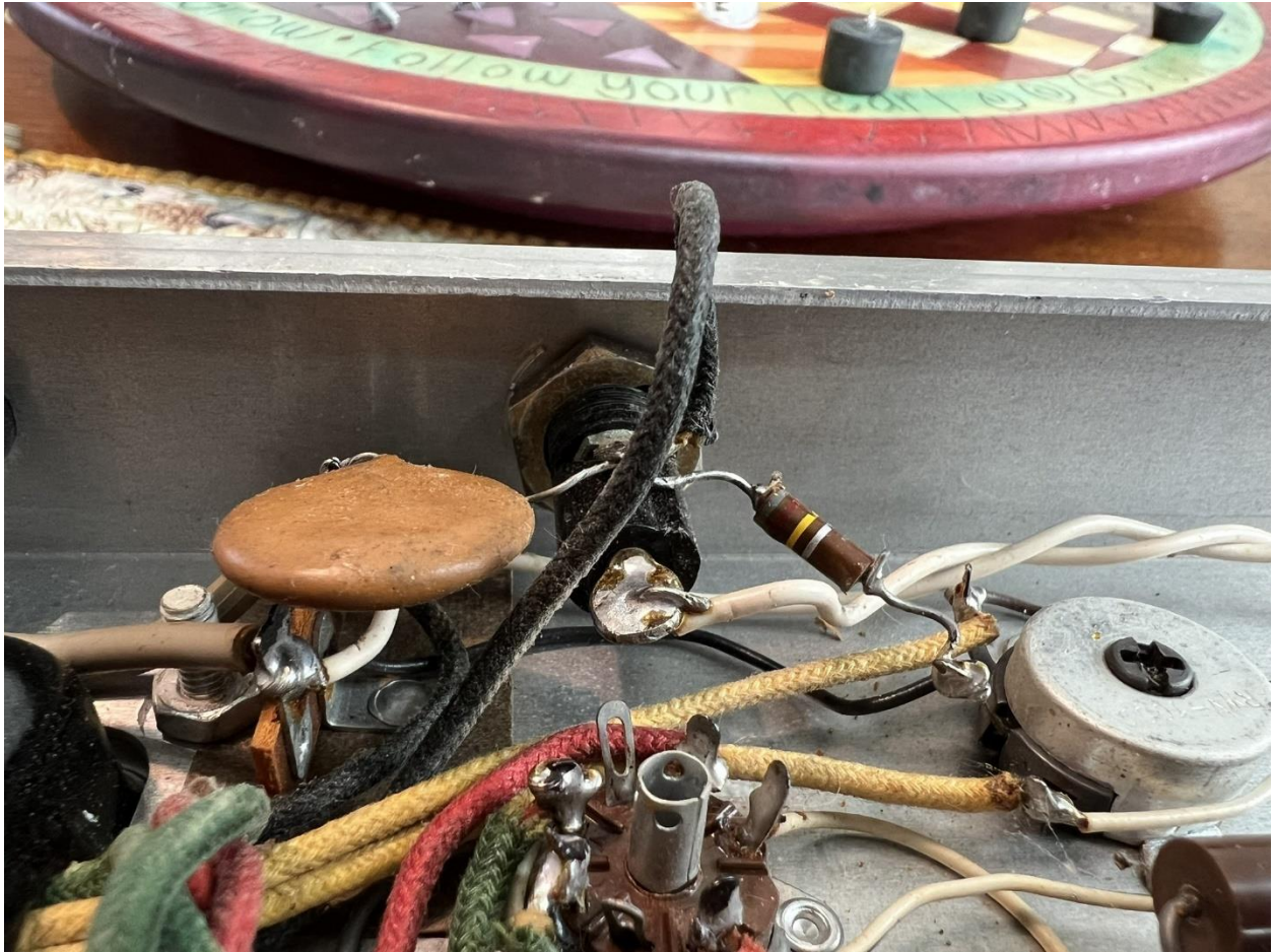
Figure 2: C2 removed; it was in parallel with the resistor.
