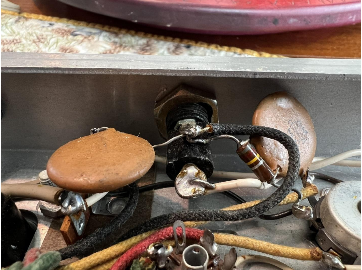
Figure 1: Tuner upside-down on workbench. C2 is the right of the fuse holder, C1 to the left.
