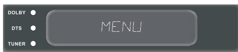
The front panel display of the LMC-1 will indicate most all of the same menu choices as the OSD, but longer selections will scroll from right to left
