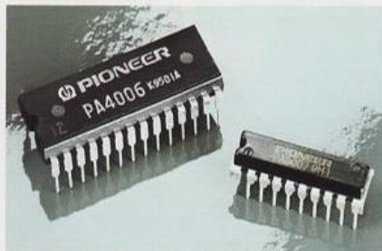
QUARTZ-SYNTHESIZER section has an independent LSI
