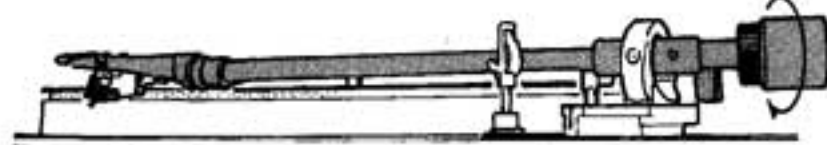
Fig. 13-A: Headshell end heavy — turn counterweight in direction of arrow.
