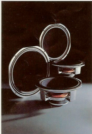
Heavy die-cast aluminum woofer frames and dual surrounds minimize resonances and coloration. Mass-loaded passive radiators augment output at lowest frequencies.
