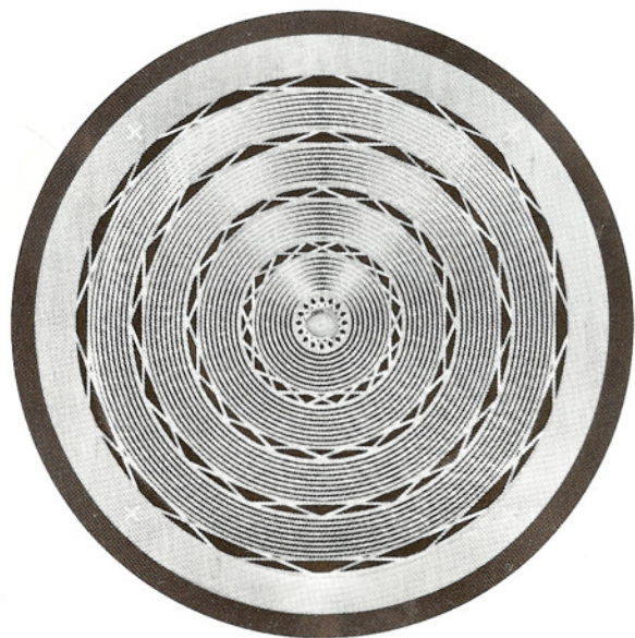
Constant Energy Orthodynamic diaphragm.
