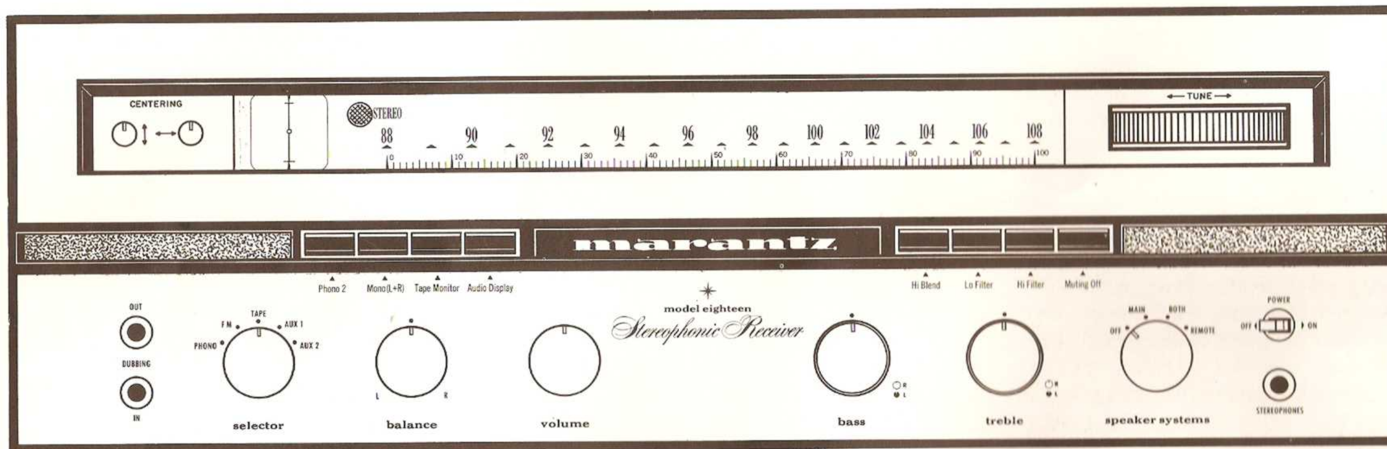
Figure 9. Front Panel Controls, Jacks, and Display CRT
