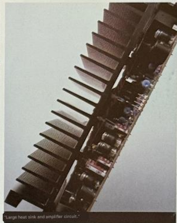
Large heat sink and amplifier circuit.
