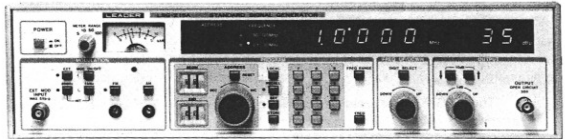
Fig. 8-6 Setting of the LSG-215A for measurement of AM practical sensitivity
