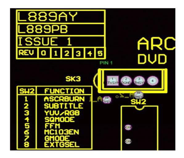
Diagram 2 – points to solder to on DSP board
