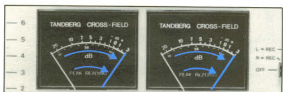
Distortion may occur if the pointers pass too far into the red sectors
