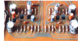
Precise 3 stage direct coupled phono equalizer on SA-7500.
