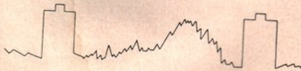
Figure 4—Normal Video and Sync Signal.
